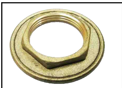
RR [ IMPORT ] RMC - B04 3/4" Brass nut Dia: 44.5mm Thick: 7.5mm
